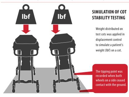
Fig. 1: Test set-up of tipping point due to side load as a result of patient weight.
